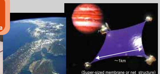
(Super-sized membrane or net structure) Furoshiki satellite
