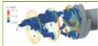
Computed large-scale recirculating eddies in impellers' inlet
