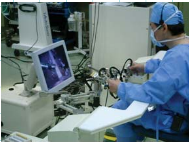
Figure: Master manipulators for internal organs of minimally invasion laparoscopy
